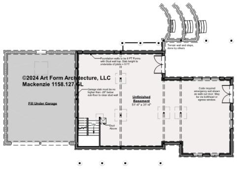
Rough Ceiling Height: 9 FT (8 FT Form height w-pony wall top, unless noted otherwise) 9 1/2" I-joists Framing
